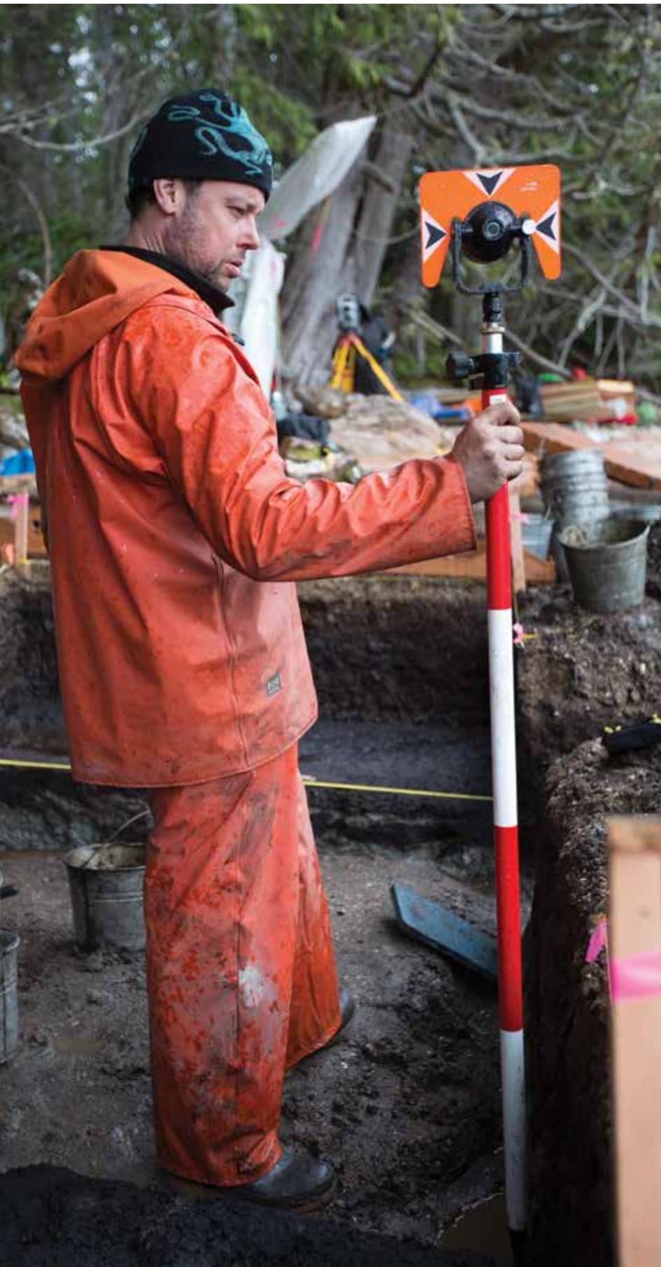
*Duncan McLaren holds a prism that's used for mapping with a total station.*
